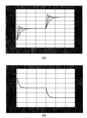
Fig. 5 Step responses with noninteracting controll [(a)  $n_e[rps]$ , (b)  $\theta_{cp}[rad]$ ).
